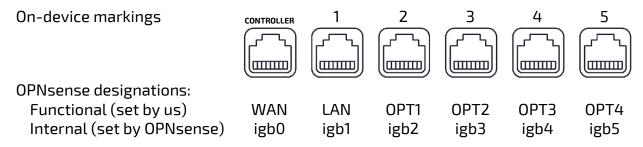
In short, the port labeled **CONTROLLER** is now the **WAN** port and port **1**, the **LAN** port. The remaining ports have been designated **OPT1** through **OPT4** but have not been configured any further.
