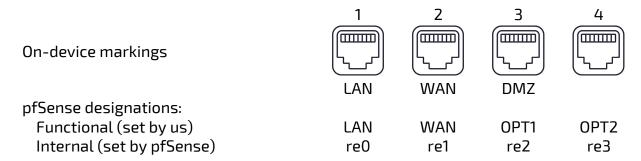
In short, the port labeled **LAN** is now officially a **LAN** port, and same goes for **WAN**. Note that if you reset pfSense to the initial state, it will by default set up **re0** as the **WAN** port and **re1** as the **LAN** port.
